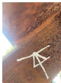
Rack 82, evidence of porosity and lack of side wall fusion.
